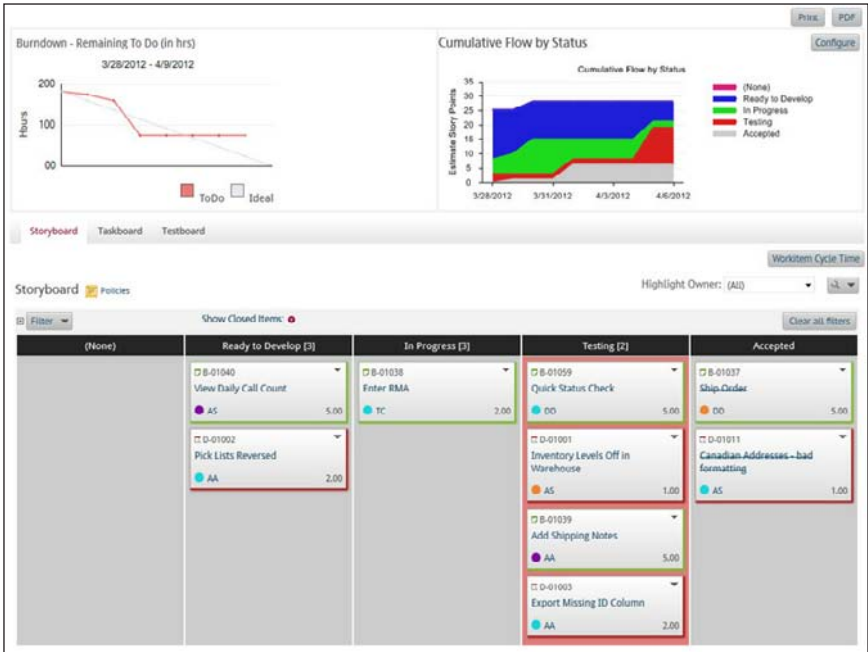
Figure 10-6 Sample task board from VersionOne agile project management tool. (Source: VersionOne, http://www.versionone.com/product/agile-project-management-tool-overview/ )
