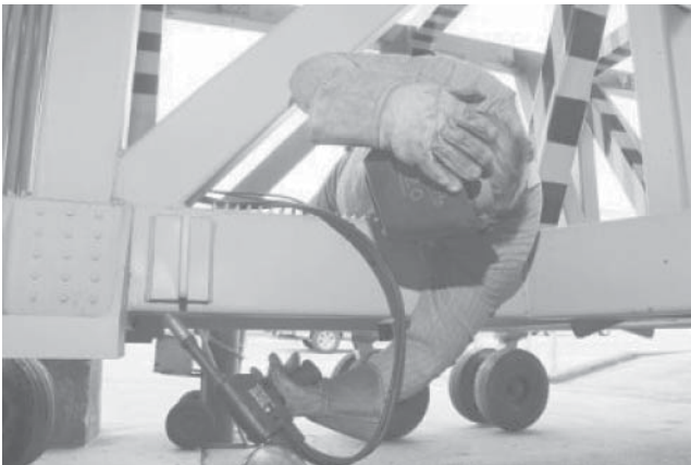
Figure B.1 Welding with the hands in front of the body. Ergonomics Stressors: Compression: Leaning on a hard surface and Awkward and Static Posture: Holding the arms away from the body for long durations (Photo adapted from Ergonomics Guide for Welders, unpublished Navy Occupational Safety and Health Working Group, Ergonomics Task Action Team with technical support provided by the Certified Professional Ergonomists at General Dynamics Information Technology (GDIT), San Diego, CA, 2010)
