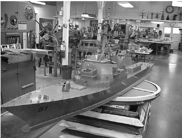
Figure 12.6 Rotating lift table used for inspection or building
