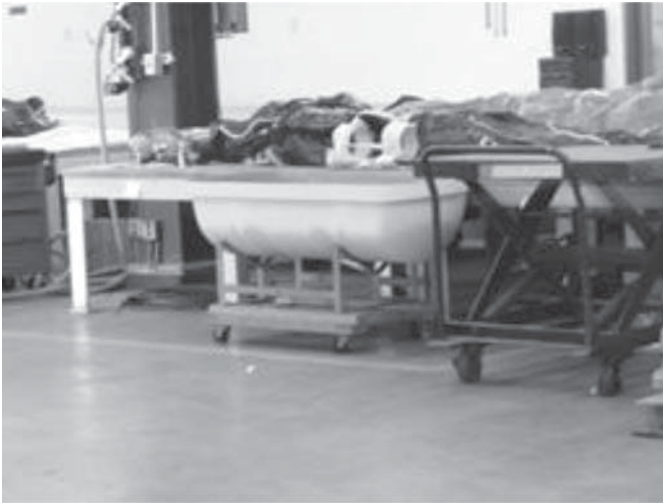
Figure 5.5 Life raft shop—elevated worktable and pod cart reduces bending to pack life rafts
