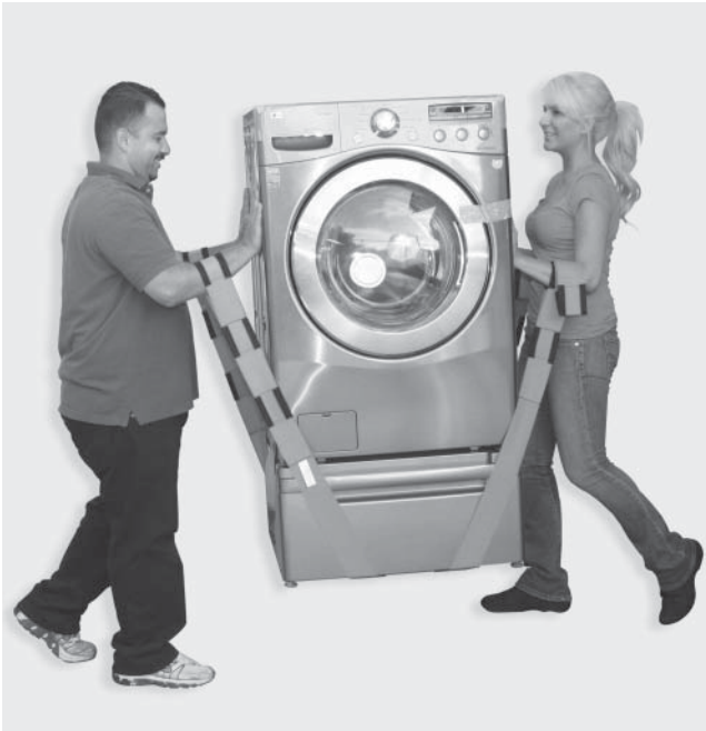
Figure 12.12 Arm lifts help the worker to maintain a neutral upright posture and eliminate compression on the hands (Adapted from www.forearmforklift.com )
