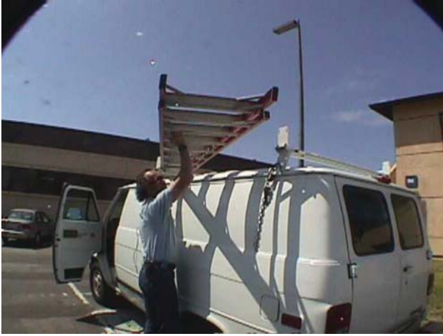
Figure 12.10 Before: Worker climbs and stretches while balancing on the ledge of a van to reach heavy ladder risking falls and soft tissue injuries
