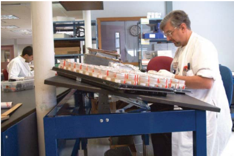
Figure 12.3 Tilting lift table orients work to the worker so they do not need to bend forward
