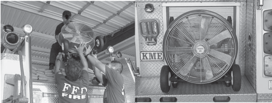
Figure 2.4 (a) Firefighter carried a heavy fan over unstable footing and lowered it to workers below. (b) Mounting the fan on the bumper eliminated the hazards
