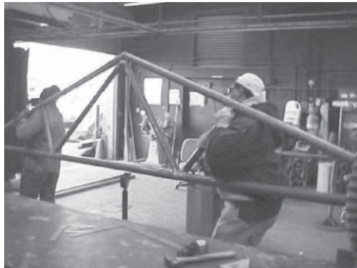
Figure B.8 Manual lifting and carrying of fabricated work piece. Possible solution, an overhead crane eliminates hazards, saves time and effort, and protects finished product (Photo adapted from Ergonomics Guide for Welders, unpublished Navy Occupational Safety and Health Working Group, Ergonomics Task Action Team with technical support provided by the Certified Professional Ergonomists at General Dynamics Information Technology (GDIT), San Diego, CA, 2010)
