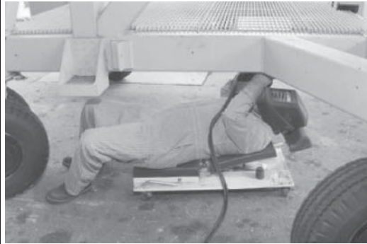
Figure B.12 After: Welder is in a supported poster and can easily see the work piece (Photos adapted from Ergonomics Guide for Welders, unpublished Navy Occupational Safety and Health Working Group, Ergonomics Task Action Team with technical support provided by the Certified Professional Ergonomists at General Dynamics Information Technology (GDIT), San Diego, CA, 2010)
