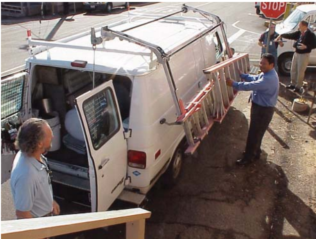
Figure 12.11 After: Worker safely removes ladder from curb side
