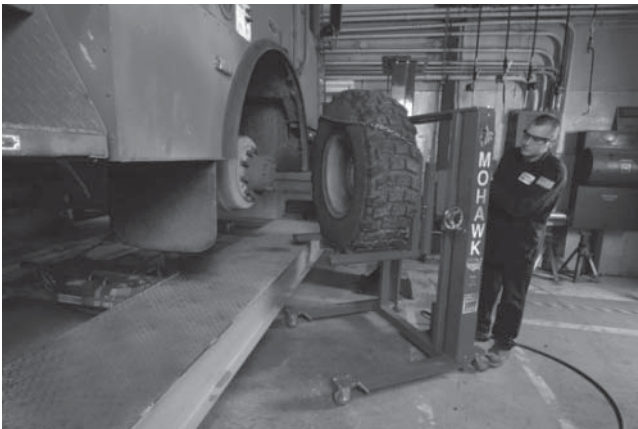
Figure 1.2 After the intervention, a tire dolly does much of the manual labor (Photo courtesy of www.mohawklifts.com )
