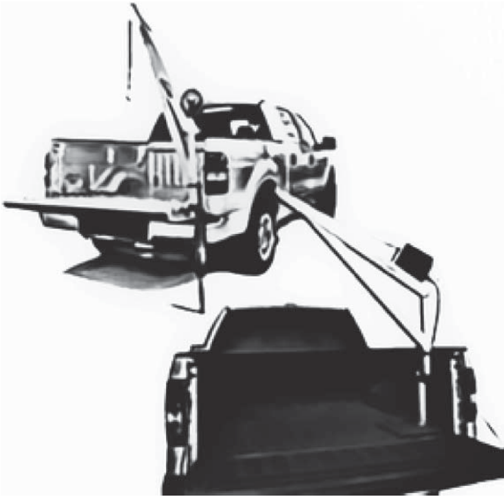
Figure 16.29 Truck mounted crane (Graphic by Lee Ostrom)
