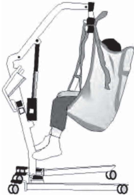
Figure 15.8 Portable lift device (sling type); can be a universal/hammock sling or a band/leg sling. (Adapted from Guidelines for Nursing Homes OSHA 3182-3R 2009)
