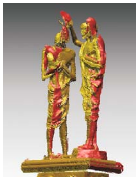
Fig. 3 Wrong registration of merged scan groups
