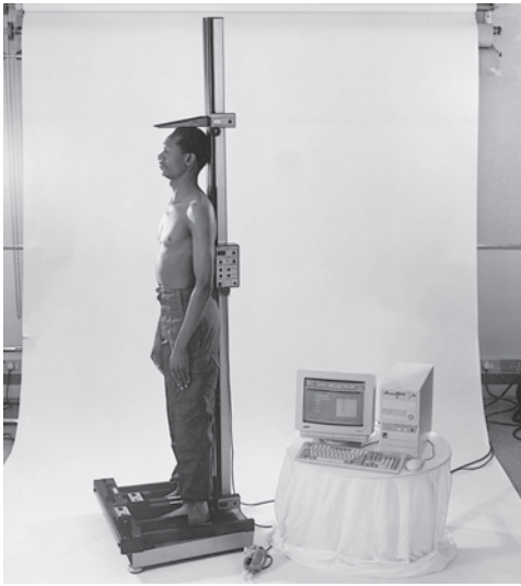
Figure 3.1 Semi-automatic capture of anthropometric data. Variables are measured using digital caliper and tape measure and automatically entered into a computer according to a pre-planned measurement protocol. (Photograph courtesy of Ergotech Consultants, Pretoria, South Africa.)
