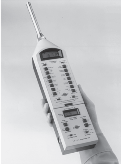
Figure 11.8 A modern sound level meter with octave filter set attached. (Photograph supplied by Messrs Bruel and Kjaer, Naeram, Denmark.)
