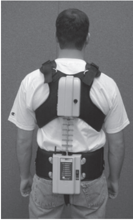
Figure 6.4 A lumbar motion monitor. (Courtesy of Professor W. S. Marras.)
