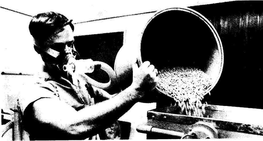
FIGURE 8-4 Apparatus for monitoring heart rate and obtaining oxygen consumption levels of a person while working on the job. (Photograph courtesy of Human Factors Department of Eli Lilly and Company.)
