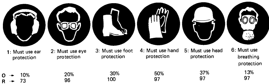
FIGURE 4-16 Symbols of mandatory-action messages used in a study of recognition and recall of such symbols. The percentages below the symbols are the percentages of correct recognition, as follows: O = original test; R = recall 1 week later. (Source: Adapted from Cairney and Siess, 1982, Fig. 1.)
