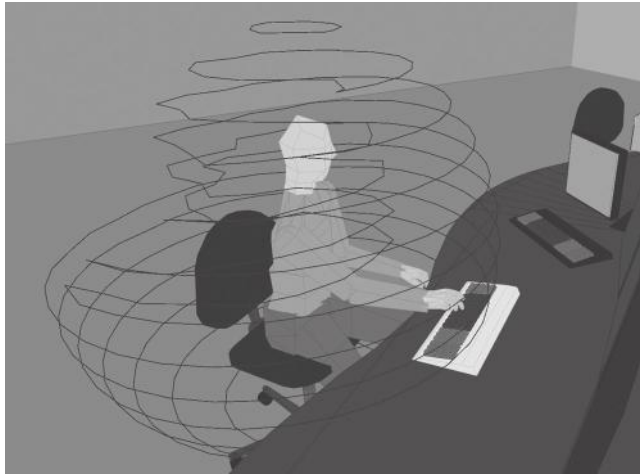
FIGURE 20.7 A DHM with a reach envelope for the right arm in SAMMIE.
