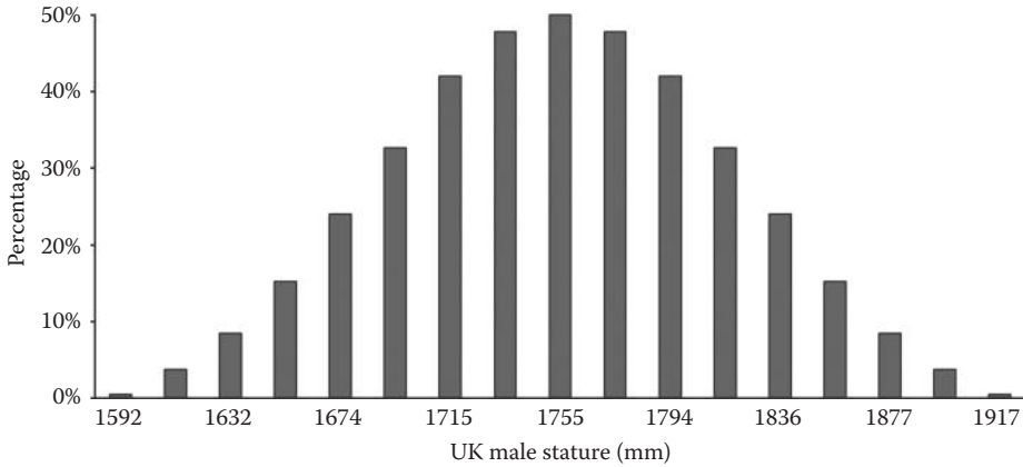
FIGURE 20.3 Stature of UK males showing a typical normal distribution. (Data from ADULTDATA, The Handbook of Adult Anthropometry and Strength Measurements – Data for Design Safety , Department of Trade and Industry, London, 1998.)
