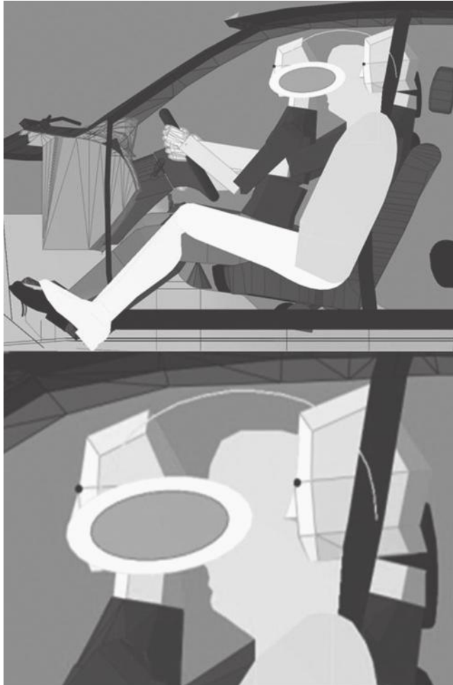
FIGURE 20.14 A comparison between the SAE eye location data and the eye points found for a 95th percentile U.S. male and a 10th percentile U.S. female.
