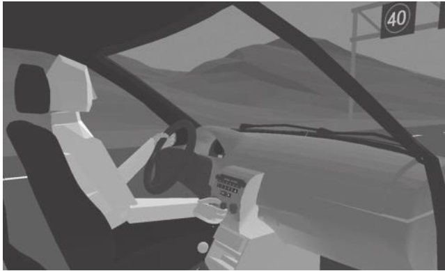
FIGURE 20.15 The car model in the SAMMIE DHM system with a small female driver interacting with the HVAC controls.
