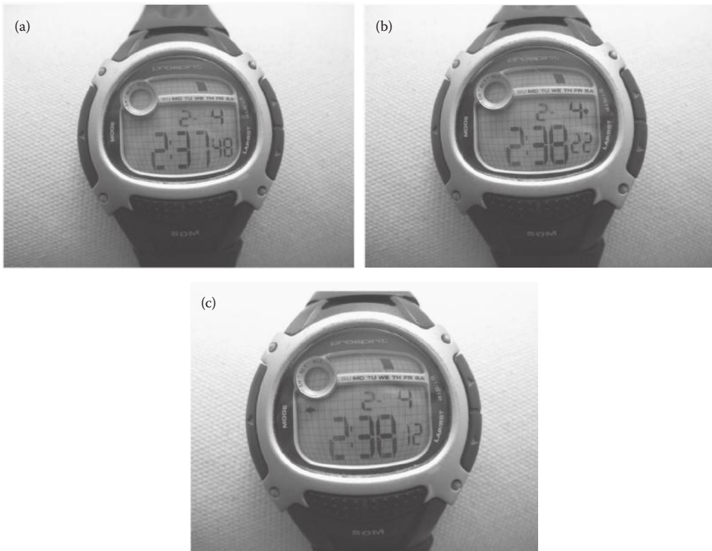
FIGURE 6.1 Three steps in setting time on a digital watch—note how the watch guides the user through the interaction by arrows on the display pointing to the next button press.
