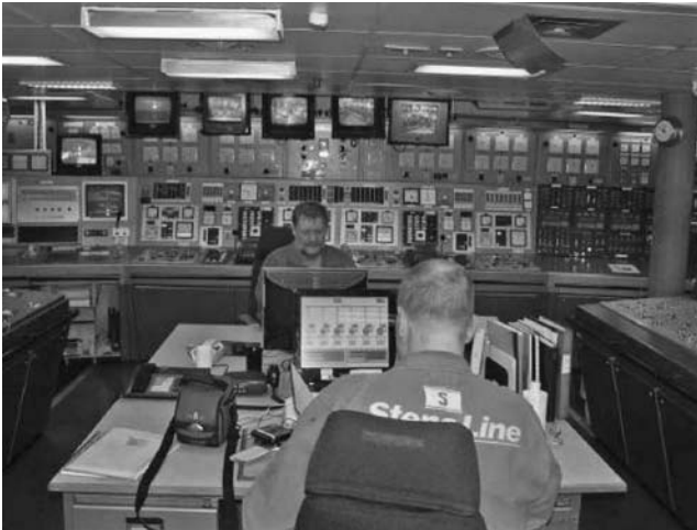
FIGURE 9.17 A traditional design of an ECR using analogue techniques. The on-duty engineers are located centrally and have a good view of the operational status and the alarm status. (Personal photograph of M. Lundh.)
