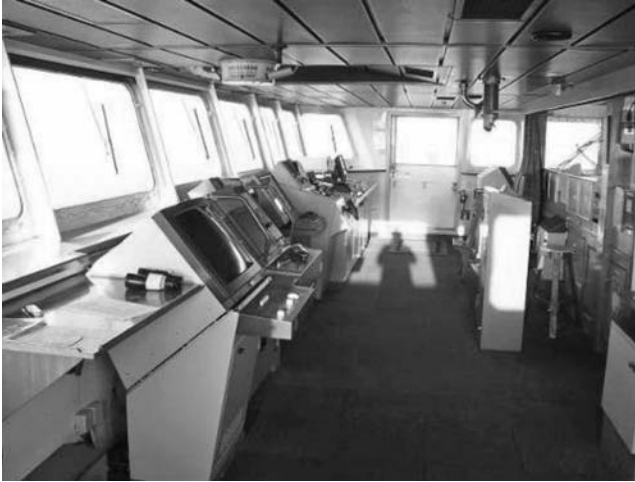
FIGURE 9.7 Traditional long console bridge, view from the port to starboard side. (Personal photograph of M. Lundh.)
