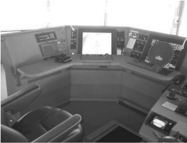
FIGURE 9.9 A modern bridge with fixtures and fittings that can be adapted to different needs. (Design by Wallenius Marine AB/Furuno Finland. Photograph used with permission.)
