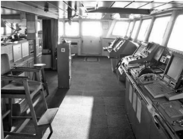
FIGURE 9.6 Traditional long console bridge, view from the starboard to port side. (Personal photograph of M. Lützhöft.)
