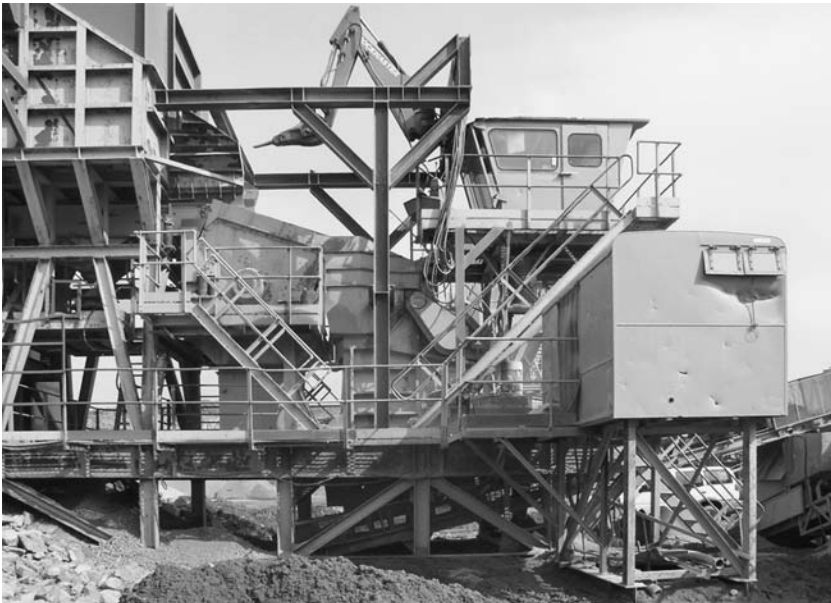
FIGURE 7.10 Control room mounted on a primary crusher in a quarry. The WBV-weighted vibration on the floor of this control room exceeded 1.15 \text{ ms}^{-2} on one axis. (Photograph by A. Nicholl.)
