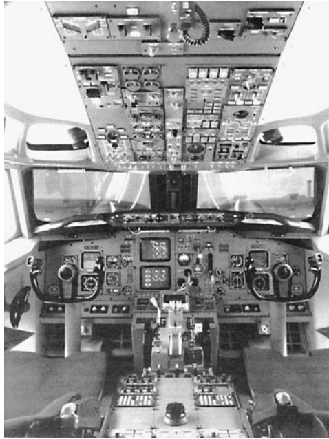
FIGURE 19.3 Boeing 737 simulator cockpit installed on motion-based platform shown in Figure 19.2. (Courtesy of Frasca Corporation.)
