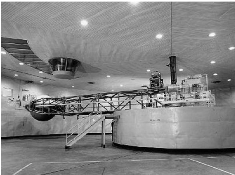
FIGURE 19.5 Dynamic flight simulator and centrifuge arm. (Courtesy of Naval Air Warfare Center, Aircraft Division.)
