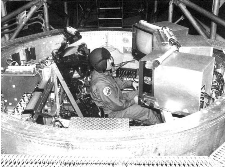
FIGURE 19.6 Cockpit installed in gondola of DFS (the top and bottom portions of the gondola have been removed). (Courtesy of Naval Air Warfare Center, Aircraft Division.)
