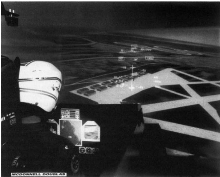
FIGURE 19.1 Generic tactical aircraft simulator installed in a dome. Note high-quality imagery immediately forward of the “nose” of the simulator. (Courtesy of McDonnell Douglas Corporation.)
