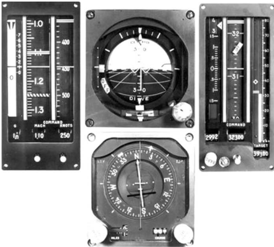
FIGURE 15.1 Integrated instrument panel showing the T-line concept.
