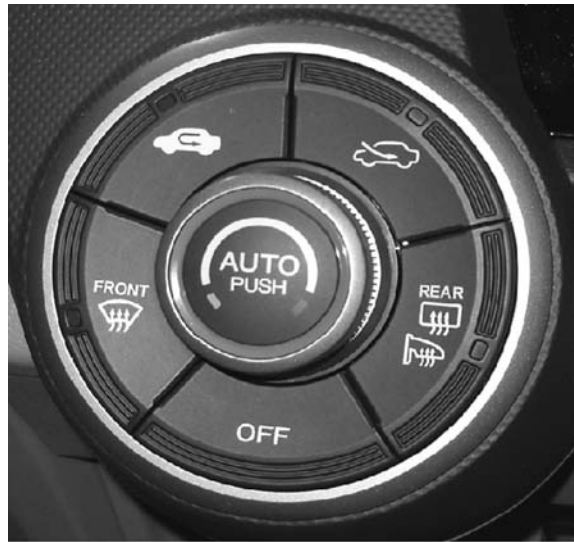
FIGURE 5.3 Rotary temperature switch with a push button in the middle (to set auto climate control) and surrounded by five push buttons to select modes for a climate control.
