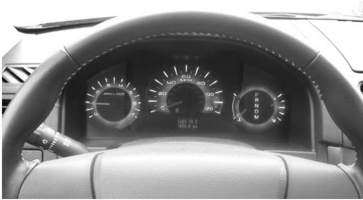
FIGURE 5.5 Instrument cluster located within obscuration-free area between the steering wheel rim, spokes, hub, and the turn signal stalk.
