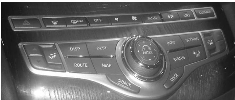
FIGURE 5.4 A multifunction rotary switch (in the middle) that can be rotated as well as moved in different directions like a joystick.
