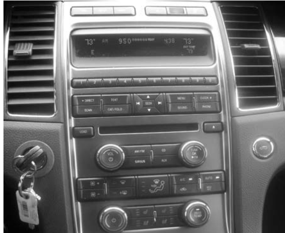
FIGURE 5.6 Functional grouping of controls in the center stack.
