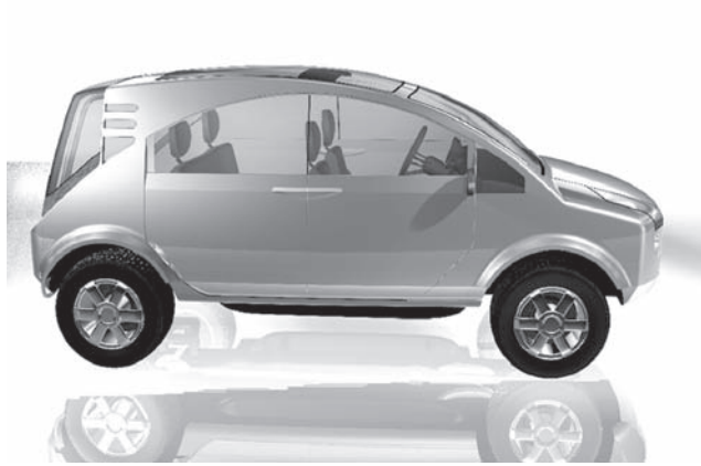
FIGURE 11.4 Fully surfaced vehicle with shading and reflections details.
