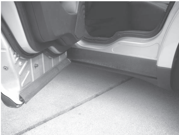
FIGURE 8.4 Hidden rocker and foot access space provided to reduce entry/exit difficulty.
