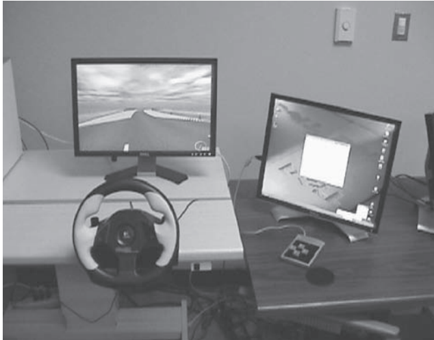
FIGURE 14.1 The laboratory setup of the LCT test showing the driver's screen on the left and the secondary task screen and controls on the right-side table.
