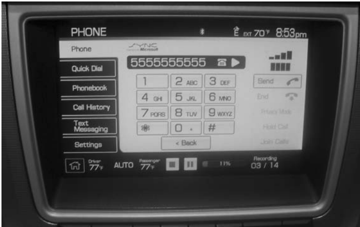
FIGURE 5.2 Touch screen with controls overlaid on the display surface.
