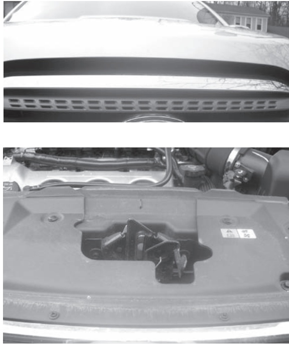
FIGURE 9.1 Illustration of difficulty in finding the secondary hood release lever. (The top picture shows the partially open hood, which does not allow good visibility of the hood release handle. The bottom figure shows the inside hood release lever that is located over 100 mm deep from the edge of the hood and thus requires a palm insertion of about 125 mm to activate the lever.)
