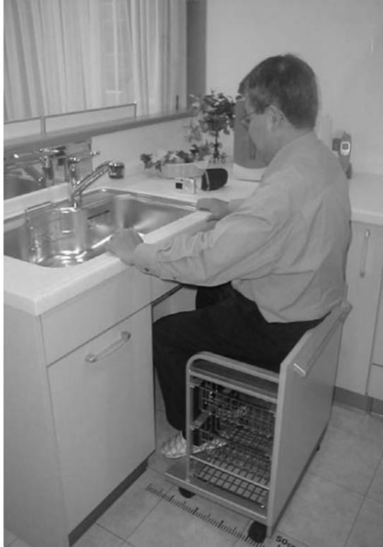
FIGURE 4.3 Junichi Hashimoto, an Edmonton architect, demonstrates use of roll-in seat at kitchen sink located in Hokkaido's Asai Gakuen University Universal Design Show Home. (Photo taken by Liu, L., 2004.)
