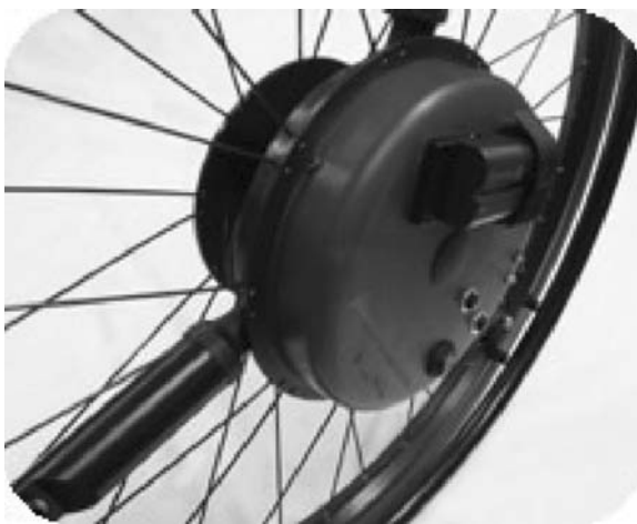
FIGURE 6.6 The Smartwheel, a six degrees of freedom force-sensing measurement hand rim wheel.
