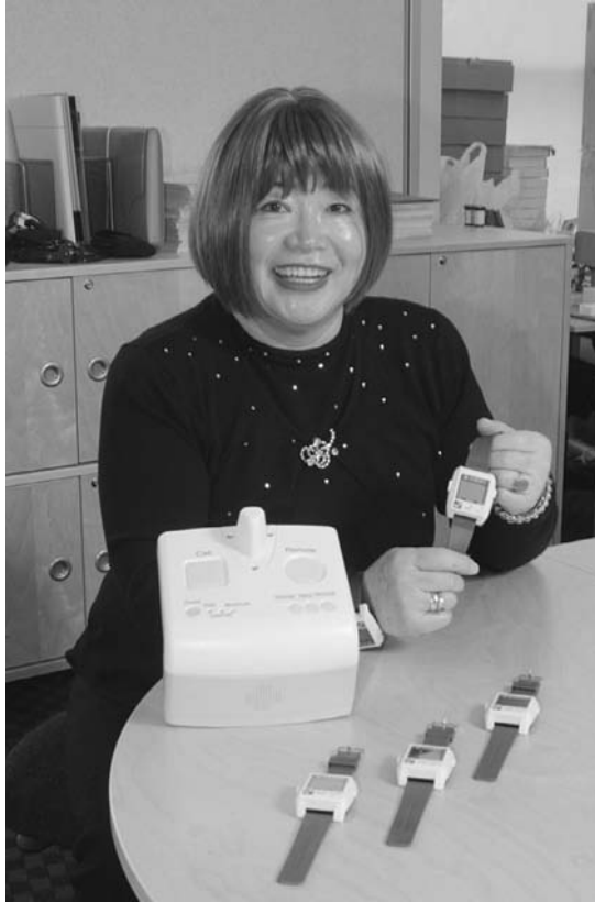
FIGURE 4.12 Dr. Masako Miyazaki demonstrates the size of the WPS which is worn on the wrist like a watch, and the WS, which uses Bluetooth to transmit data to a central server. (Photo by Bourque, T., Edmontonians , March 2006.)
