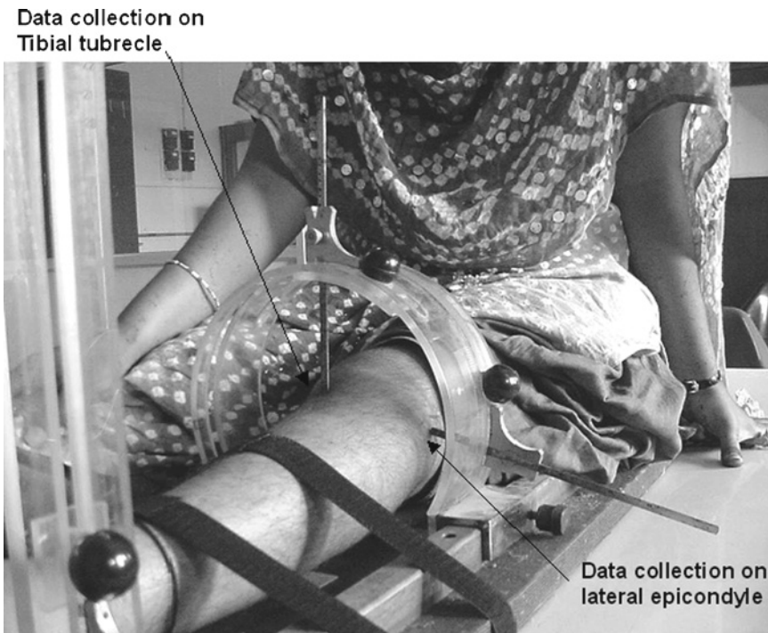
Fig. 47.3 Data collection on knee in an anthropometric device. (Reproduced from Dwivedi et al. 2009)
