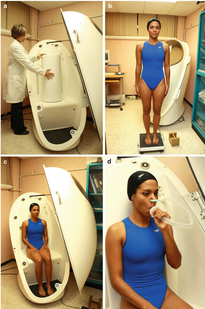
Fig. 22.3 Sequence for the measurement of body volume using ADP (courtesy of CIAD, Mexico). (a) The instrument is calibrated before a series of measurements using a known volume or “phantom.” (b) The individual is weighed in the calibrated scale. Note that the person is wearing tight clothing and a swimming cap, with no jewelry. (c) After a second calibration with the phantom, the individual enters the instrument and sits still. The measurement starts after closing the chamber and is performed twice. (d) To measure the lung volume, the person is instructed to breathe normally through the tube attached inside the instrument. The measurement is performed twice after the chamber is closed. The instrument will then calculate the final results
