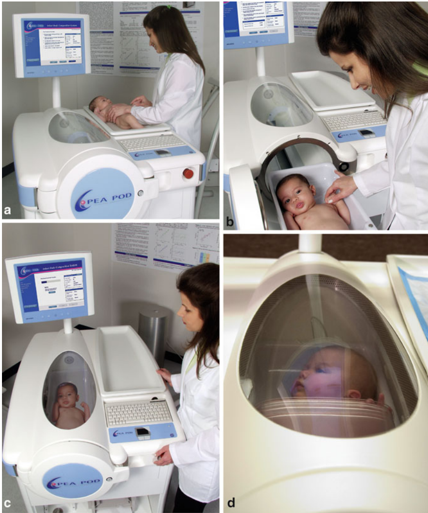
Fig. 22.5 Sequence for the measurement of body volume in infants using ADP (used under license of LMI Inc., Concord, California). (a) The infant is weighed, and at the same time, the volume of the chambers is calibrated automatically. (b) The test chamber door opens; the infant is placed in the sliding tray, and pushed into the chamber. (c) The measurement begins when the door is closed. After 2 min, the door opens and the test is completed. This procedure is performed twice. (d) The acrylic window allows the infant to be observed at all times. The behavioral state of the infant (quiet, alert, awake and active, crying, etc.) does not affect the fat % estimate (Ma et al. 2004)
