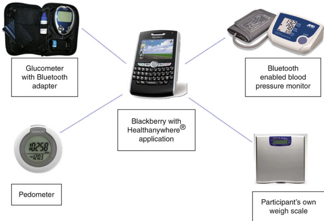
Fig. 116.4 Devices provided to participants of the DaTA pilot study. This figure shows the devices used for home monitoring of cardiovascular risk factors in the DaTA pilot study. Bluetooth-enabled glucometer and blood-pressure monitor were used for twice daily blood glucose and thrice weekly blood pressure evaluation, respectively. Pedometer was used to monitor daily activity with step count and the weigh scale was used to monitor weight weekly. All measurements were entered into the Blackberry and automatically sent to a secure database to be monitored by researchers
