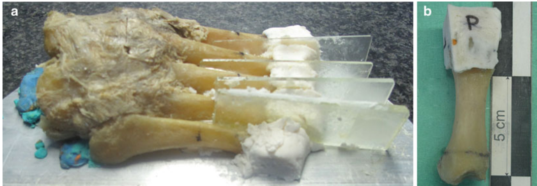
Fig. 184.17 Preparation of alignment pots for the metatarsal bones. Portion of a right foot including selected tarsal (cuneiforms, cuboid, and scaphoid) and all metatarsal bones: (a) The distal extremity of each metatarsal bone is included in bone cement while resting on a flat surface; (b) First metatarsal, after complete dissection: the flat pot on the distal extremity provides alignment about the long axis of the bone in the subsequent steps
