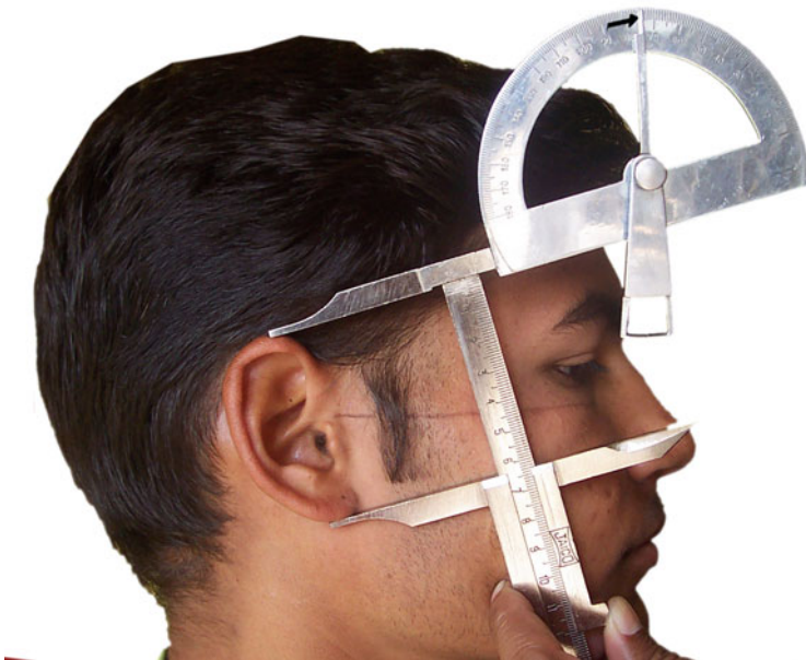
Fig. 53.4 Measuring ear inclination angle. The angle is measured with a goniometer fitted on a sliding calliper. The arrow shows the reading on the goniometer, which is 14°
