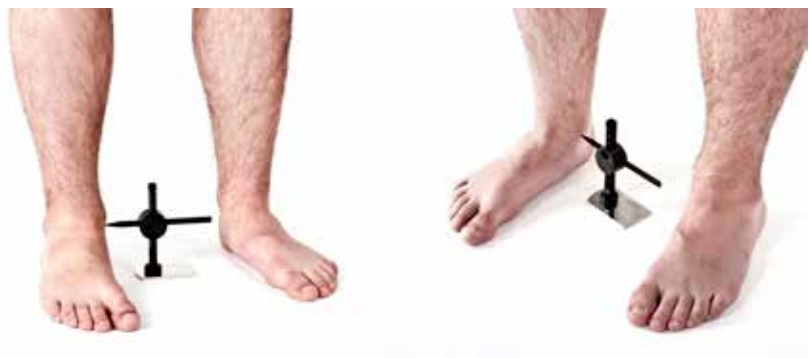
V-372 Small height rod – application in measuring the sphyrion height
