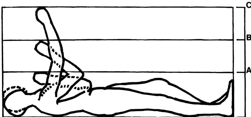
Figure 95 Inspection clearances Lying positions for inspection and repair. Minimum heights are given; the length is 1930 mm (76 in.) A Lying for inspection Height 457 mm (18 in.) B Restricted space for small tools and minor adjustments. Power from elbow extensions not possible. Height 610 mm (24 in.) C Space for reasonable arm extension 152 mm/203 mm (6 in./8 in.) length; power tools could be used. Height 813 mm (32 in.)
